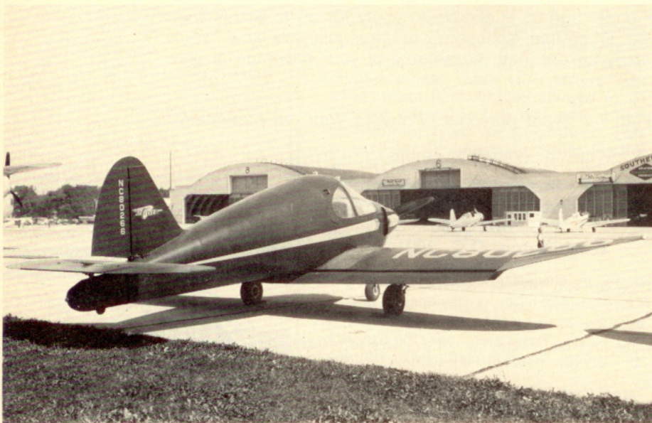
The flaps of the Culver V ran clear under the fuselage. It was a long step from the ground over the flap and onto the walkway on the wing. Note the "up" position of the horizontal tail.
