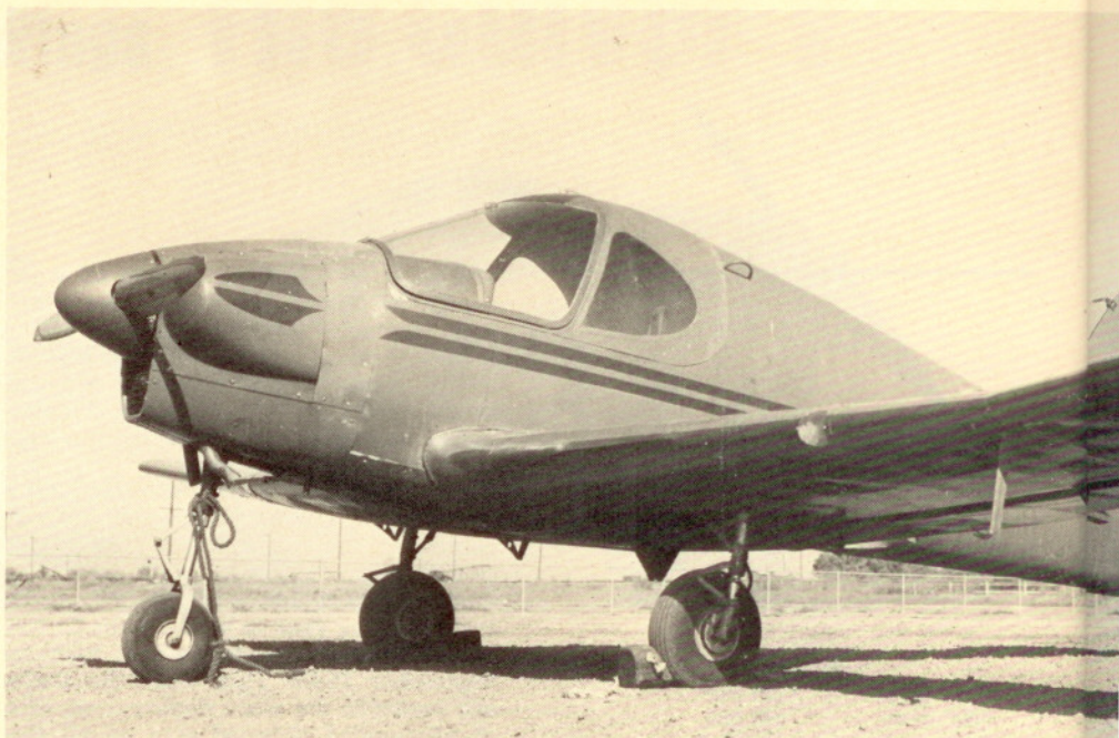
The Culver V-2 squared off the wingtips, enlarged the ailerons, shortened the flaps, and deleted such refinements as the recessed handgrips.
